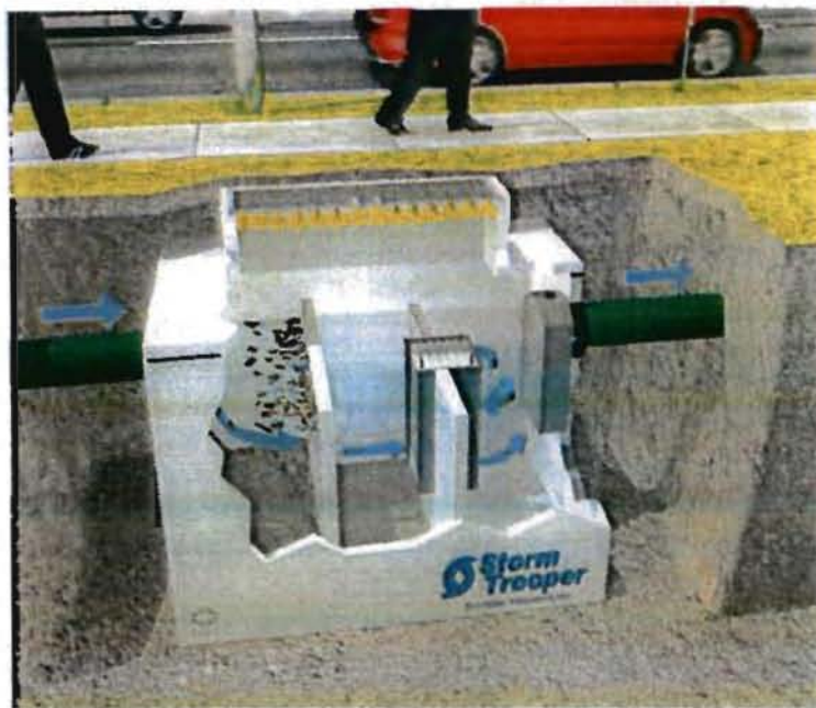
Figure 1. The StormTrooper® Stormwater Separator
