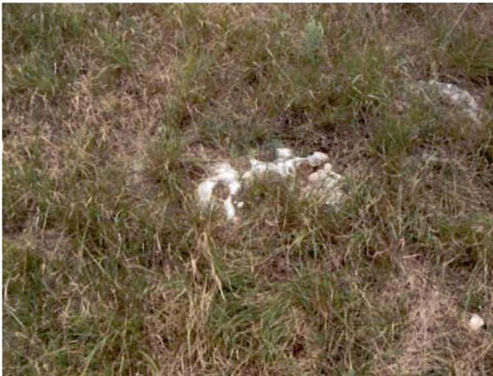
Photograph 2: Small outcrops of vuggy limestone are present on the Site, but no voids were observed.
