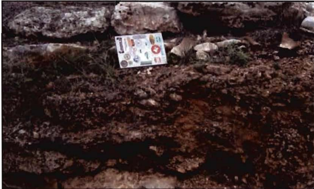
PHOTO E2 - Limestone (Kk) exposed in ROW by cut/grading to create runoff channel in ROW, paralleling FM-306. Channel in foreground. Note weathering of limestone and resulting terra-rosa soil infilling.
